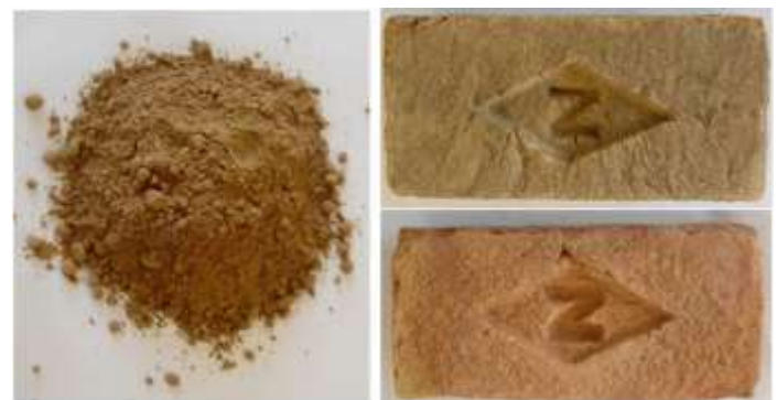
Figure 4. Clay used for bricks, dried bricks and fired bricks
